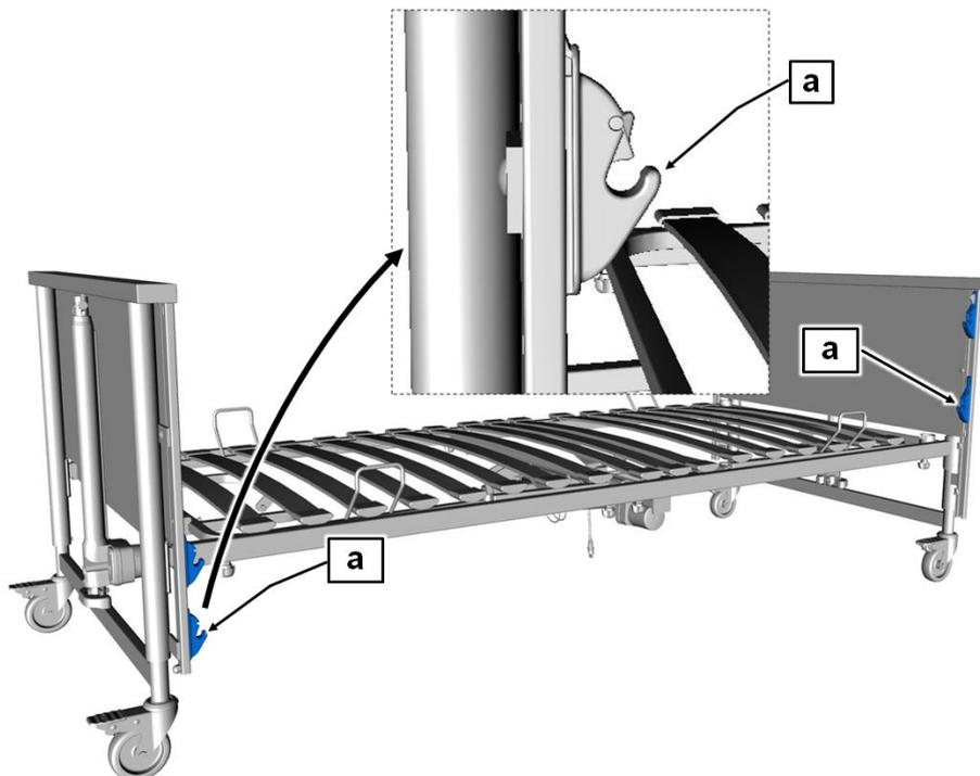
**Important:** The guide rails must be diagonal to each other before starting the assembly work (see picture). To ensure this, raise the guide rail at the head end and lower the guide rail at the foot end.
