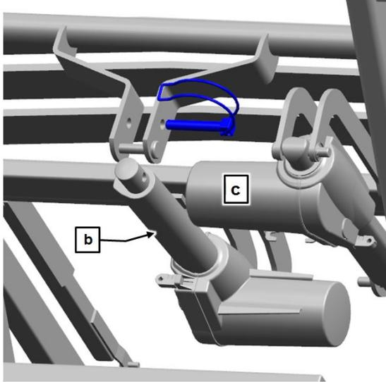
7. Insert the pin again from the side of the thigh rest motor [c]. .
