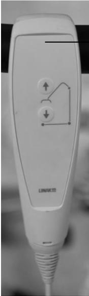
1. **Raise the lift arm** – When this button is held pressed, the lift arm moves upwards. Release the button to stop the process.
